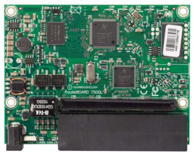
You can download the board dimensions and case design files (PDF and DXF) from www.routerboard.com
